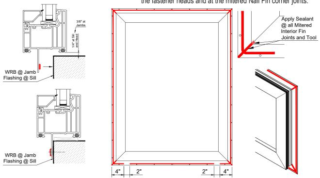
After Installing the window, apply the D313 Head and D319 Sill Flashing. Fasten in place, then securely seal over fastener heads and between the flashing and windows as shown below. Also, plug and seal the gap between the head flashing and window frame at the open ends. Tool as neeeded.
