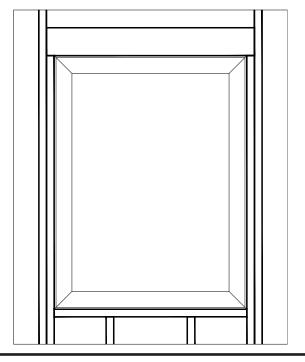
Apply a generous amount of sealant around the entire Nail Fin as shown in the sketch, leaving (2) 2" voids no more than 4" from jambs at the sill. Make sure placement of sealant will contact the LBA.
