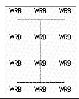
Fold the WRB sides towards the interior and trim as needed. Do not staple in place. Make 4"-6" horizontal cuts in the WRB at the head and sill jambs. Make a 45° x 6" long cut at the head condition. Fold back WRB at the cut lines, and tape into place.
