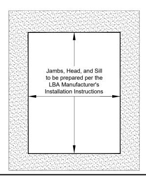
Test fit the Window Unit in the opening to ensure proper fit. Make sure unit can be installed square, plumb, and level. Insert plastic shims at the sill and jambs. The unit will come with pre-punched holes for attachment. Match drill pilot holes in the structure per the Shop Drawings or anchorage calculations. Typically, 3" from the ends and 12" on center. **NOTE:** Not all pre-punched holes will be used. When done, remove the unit.
