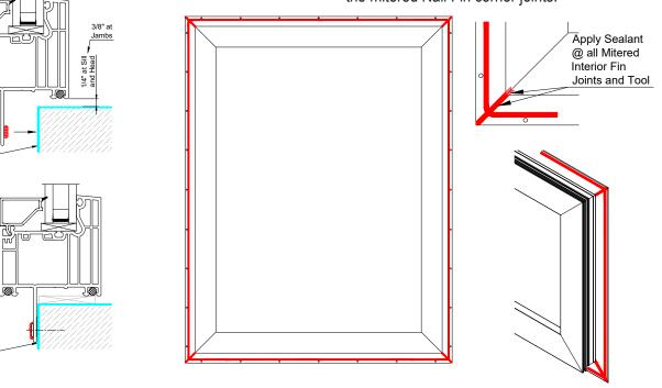
After Installing the window, apply the D313 Head and D319 Sill Flashing. Fasten in place, then securely seal over fastener heads and between the flashing and windows as shown below. Also, plug and seal the gap between the head flashing and window frame at the open ends. Tool as neeeded.
