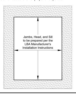
Test fit the Window Unit in the opening to ensure proper fit. Make sure unit can be installed square, plumb, and level. Insert plastic shims at the sill and jambs. The unit will come with pre-punched holes for attachment. Match drill pilot holes in the structure per the Shop Drawings or anchorage calculations.
